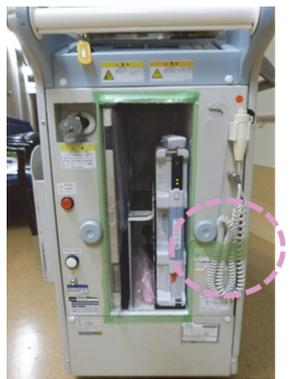
Fig.15 Curl cord suppression of exposure switches
