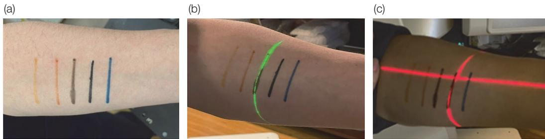
Fig.5 Visibility of skin markings drawn with a five-color marker under various conditions: Room light and illuminated laser
