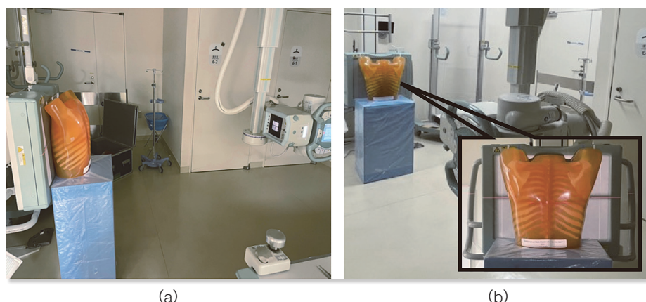
Fig.4 (a) and (b) is radiography geometry. The imaging conditions were set to frontal chest (120 kV, 3.2 mAs), and low-tube-voltage (60 kV, 3.2 mAs) images were also acquired for energy subtraction images.
