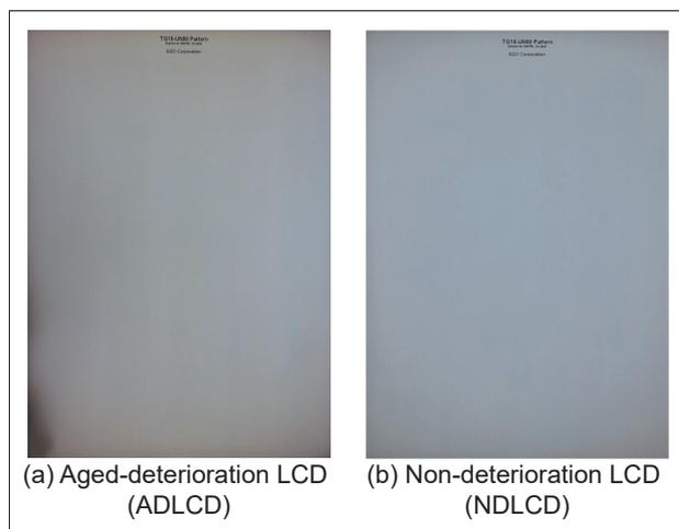
Fig.1 The same type LCDs with different operation times displayed identical uniform test-patterns. The operating times of (a) and (b) were about 38,000 and 200 hours, respectively. A luminance non-uniformity was observed for the LCD with a longer operation time.
