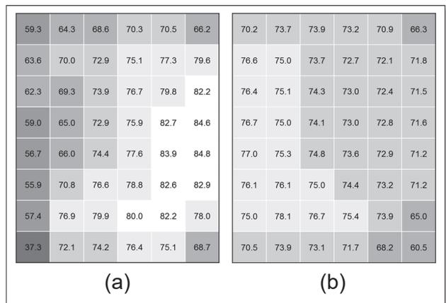
Fig.4 Luminance values (cd/m<sup>2</sup>) measured using the original test pattern (Fig.2 (b)). (a) and (b) are the luminance values corresponding to small rectangular regions of the original test pattern (Fig.2 (b)) displayed on the ADLCD and NDLCD, respectively.
