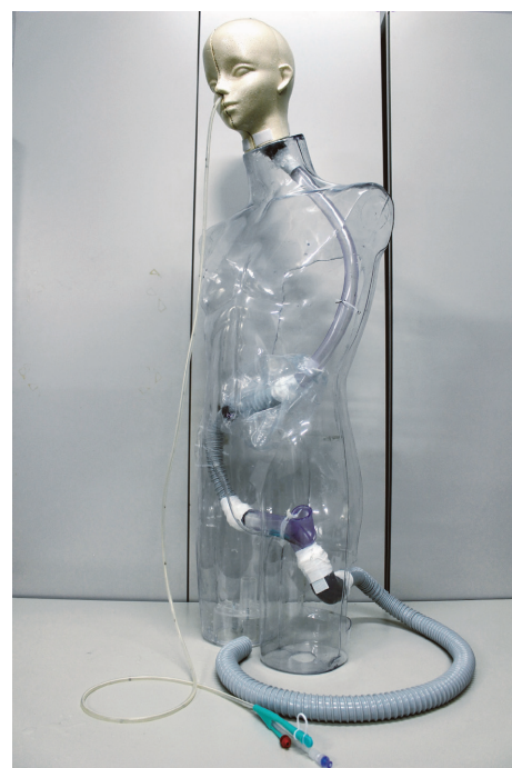
Fig.4 Whole oblique angle view of the simulator with inserted naso-intestinal catheter.
